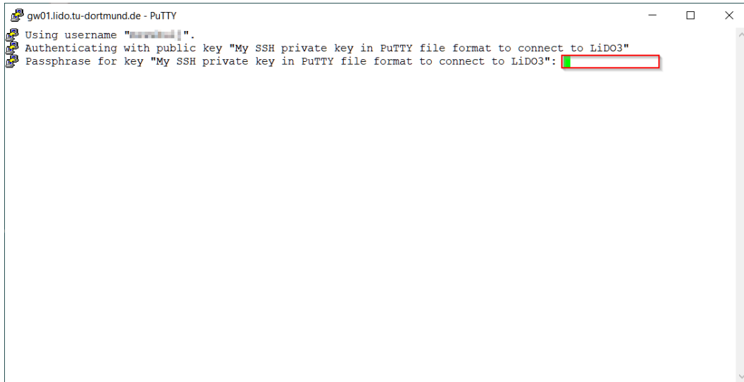
Figure 4.15: SSH private key, if you chose to encrypt it (recommended!), needs to be unlocked during login to LiDO3
